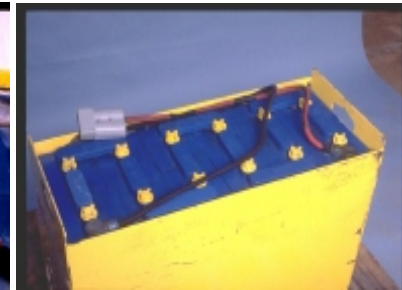
Fig. 1 An example of a poorly maintained battery. This battery will require more charge time and, as a result, less work time.
