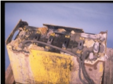
Fig. 1 An example of a poorly maintained battery. This battery will require more charge time and, as a result, less work time.
