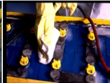
Fig. 1 An example of a poorly maintained battery. This battery will require more charge time and, as a result, less work time.
